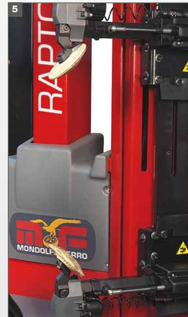
**8-9-10.** The demounting device **WITHOUT LEVER**, applied to the extraction system, **completely eliminates the physical effort of the operator and ensures maximum safety for the rim and tyre.**
