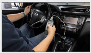
By using the radio remote control it is possible to manage the entire testing procedure. Through the same device, it is possible to transmit the forces applied to the lever (for motorcycles and three-/four-wheelers) or pedal controls to the operating program for the correct measurement of the braking efficiency.
